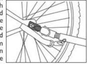
female connector on the tow bar can slide over the male connector on the hitch. Lock these connectors in place with the cotter pin. Loop the black safety strap around the bike frame and attach the snap swivel to the D-ring on the tow bar.
